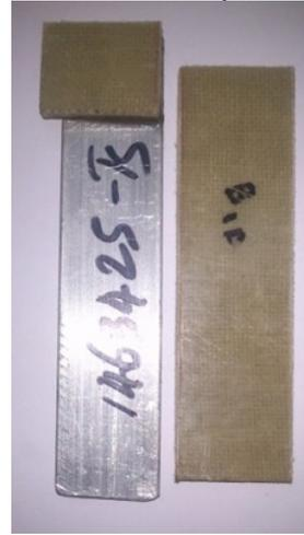
Fig. 8. Joint failed with acrylic adhesive
