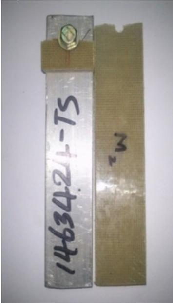
**Fig. 12.** Joint failed with mechanical fastening
