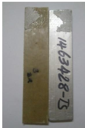
**Fig. 10.** Joint failed with rubber adhesive
