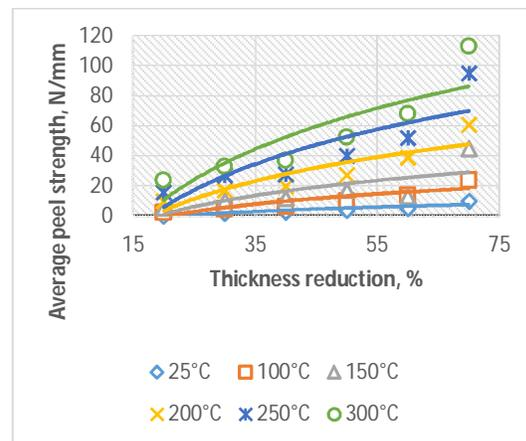
Fig. 8. Variation of the average peel strength of two-layer strips of Al/Al versus total thickness reduction at different rolling temperatures (Log-experimental).
