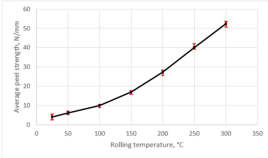
Fig. 9. Variation of the average peel strength of two-layer strips of Al/Al versus the rolling temperature.
