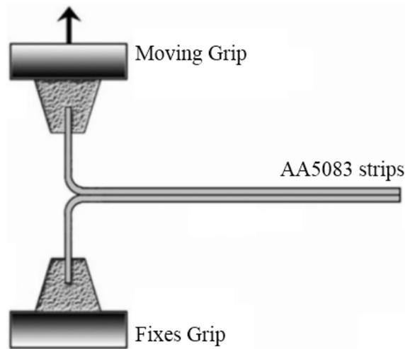
Fig. 2. Schematic illustration of the peeling test fixture.
