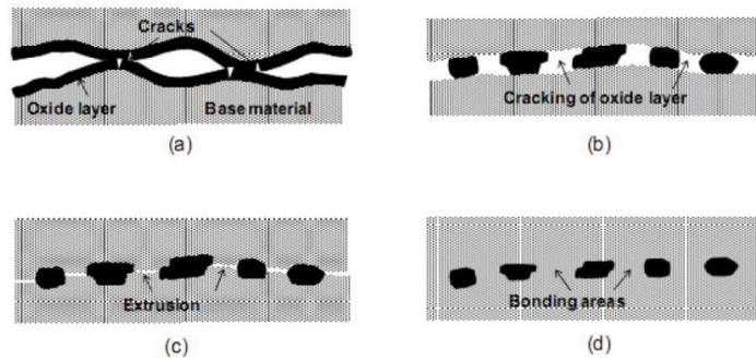
**Fig. 6.** The progression of bonding between two aluminum layers under increasing load [2].
