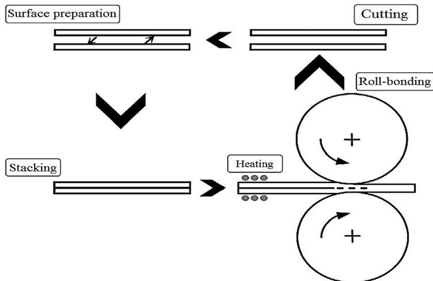
**Fig.1.** Schematic diagram of the roll bonding (RB) process.
