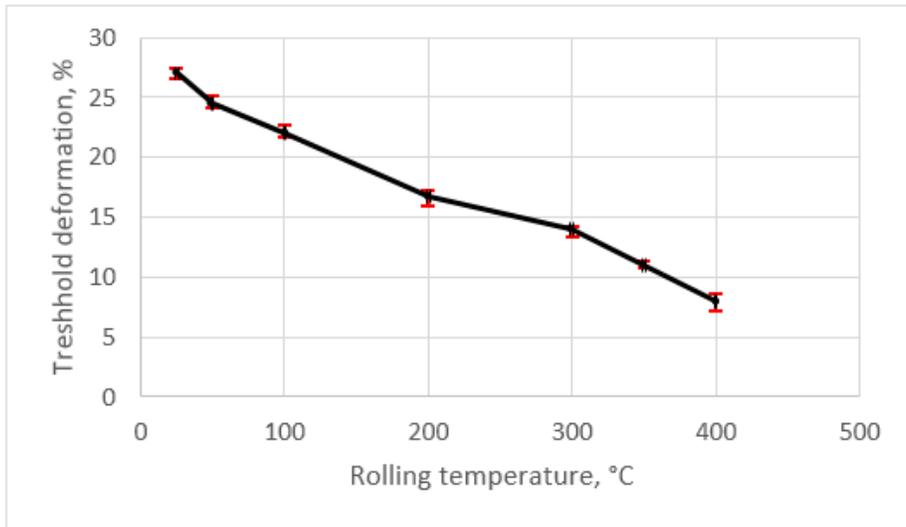
Fig. 10. Variation of threshold deformation in aluminum-1100 strips versus the rolling temperature.
