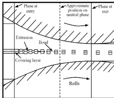
Fig. 5. Schematic illustration of the bonding mechanism in the rolling length of contact [5].
