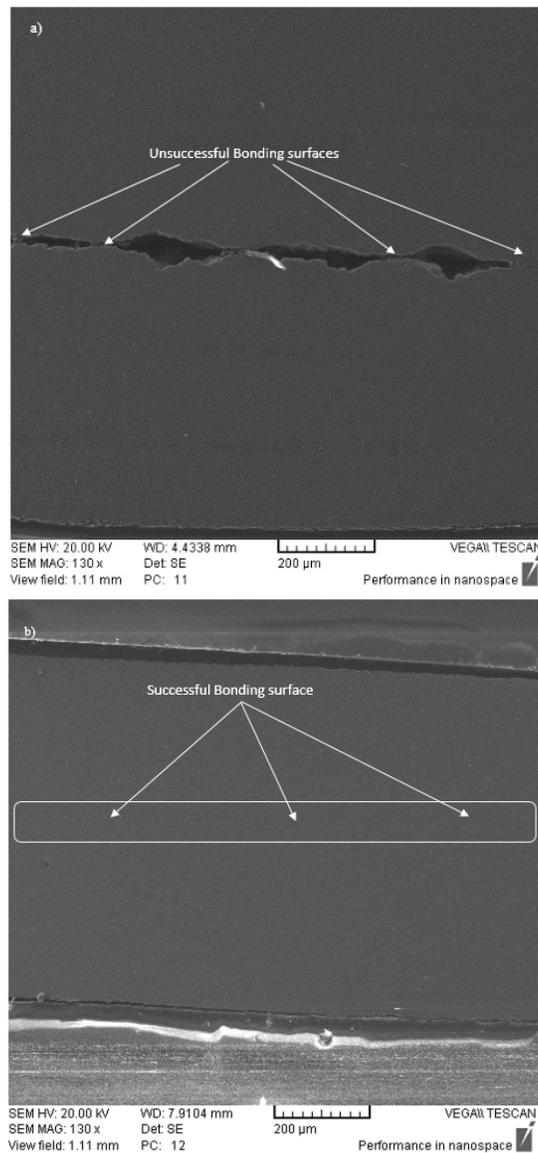
**Fig. 7.** SEM images of cross section of the samples: (a) With 10 and (b) with 70 pct. of thickness reduction at 200°C.
