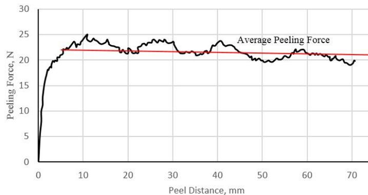
Fig. 3. Typical plot of the peeling force versus the peel distance.
