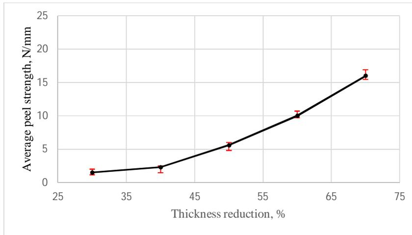
Fig. 4. Variation of the average peel strength of two-layer strips of Al/Al versus total thickness reduction.
