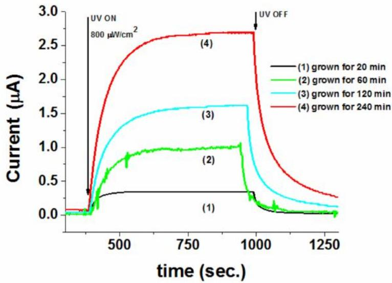
Fig.7. Ultra-violet detecting performance of ZnO nanorods grown at different times.
