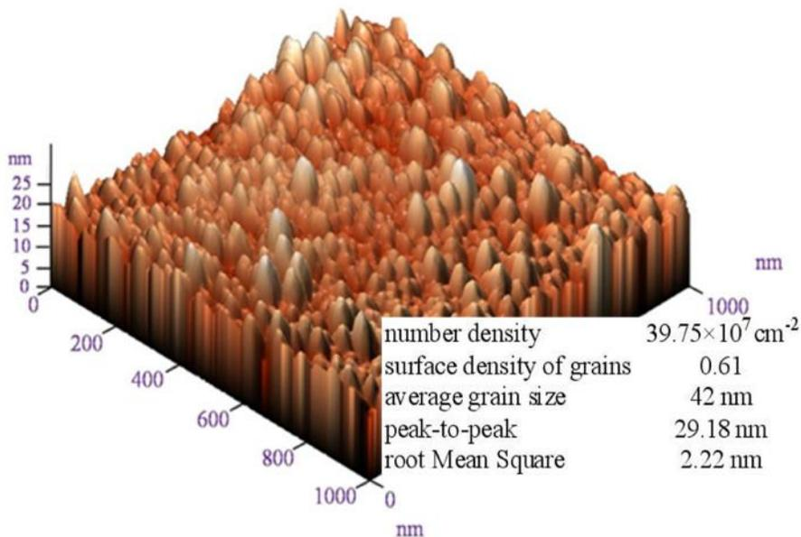
**Fig. 3.** AFM micrograph of ZnO seed layer.
