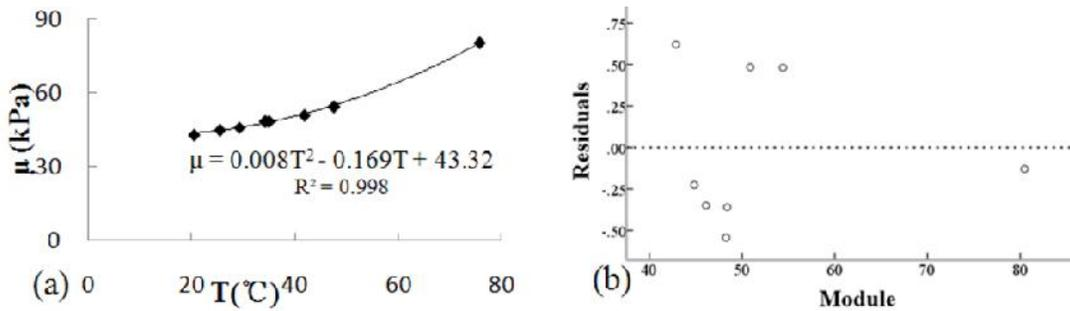
**Fig. 2.** (a) Variation of the beads shear module with the increase of temperature (experimental data (  $\blacklozenge$  ), model curve (  $\text{---}$  )); (b) Residual analysis of the model to verify the descriptive effectiveness of theoretical formula.
