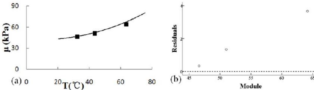
**Fig. 3.** (a) Validation of the experimental data(  $\blacksquare$  ) with the module curve (  $\text{---}$  ) of  $\mu$  as the function of temperature; (b) Residual analysis of the model to verify its predictive effectiveness.
