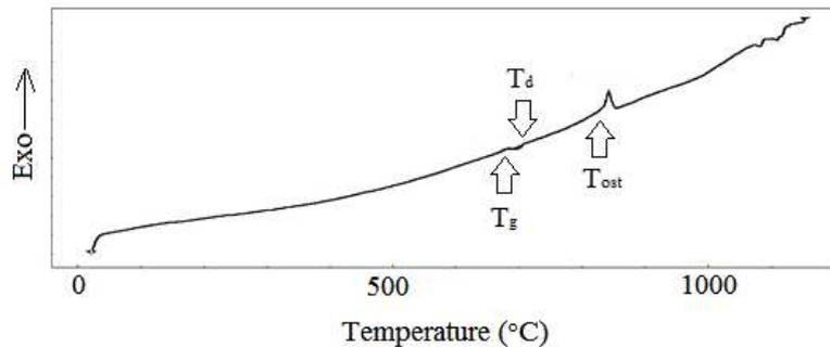
Fig. 1. DTA trace for base glass specimen
