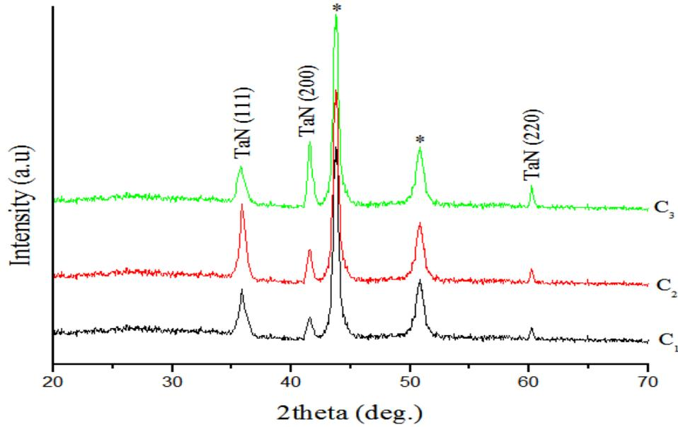
**Fig. 1.** XRD patterns of the TaN films prepared at different partial pressures of N<sub>2</sub>
