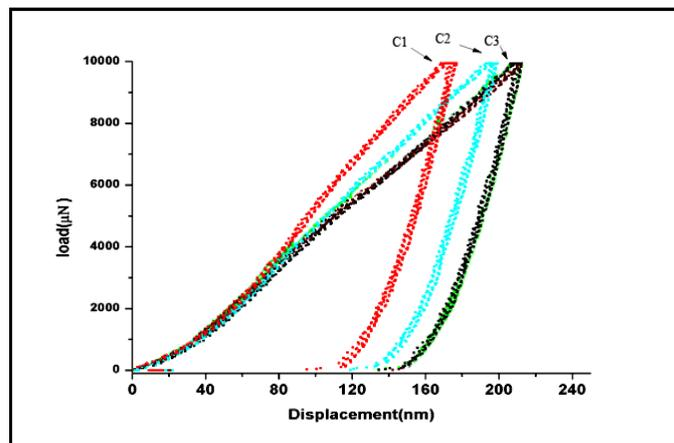
Fig. 4. Load-penetration depth curves of indentations for the TaN films with different N<sub>2</sub> partial pressures.
