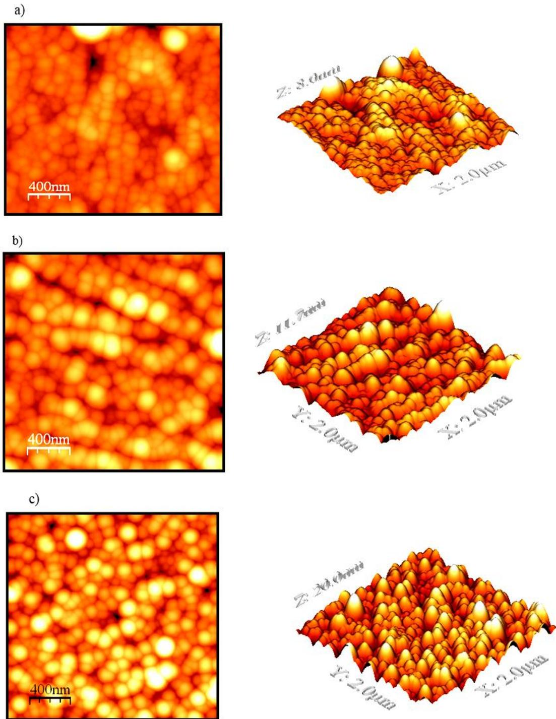
Fig. 2. AFM images of the TaN films prepared at different partial pressures of N<sub>2</sub>:(a) 10%, (b) 20% , (c) 30%.
