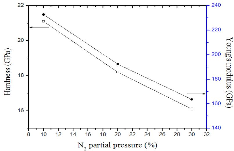
Fig. 3. Hardness and Young's modulus of the TaN films at different partial pressures of N<sub>2</sub>.
