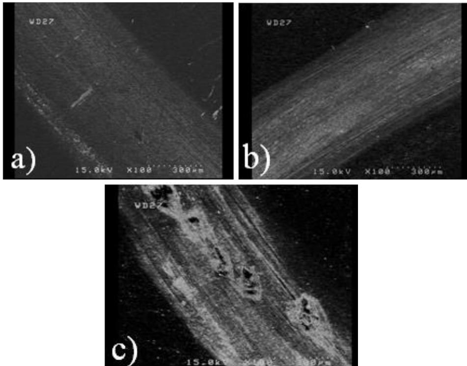
**Fig. 6.** The images of the formed wear grooves: a) sample C<sub>1</sub>, b) sample C<sub>2</sub> and c) sample C<sub>3</sub>.
