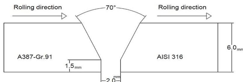
**Fig. 1.** Schematic of the joint design.
