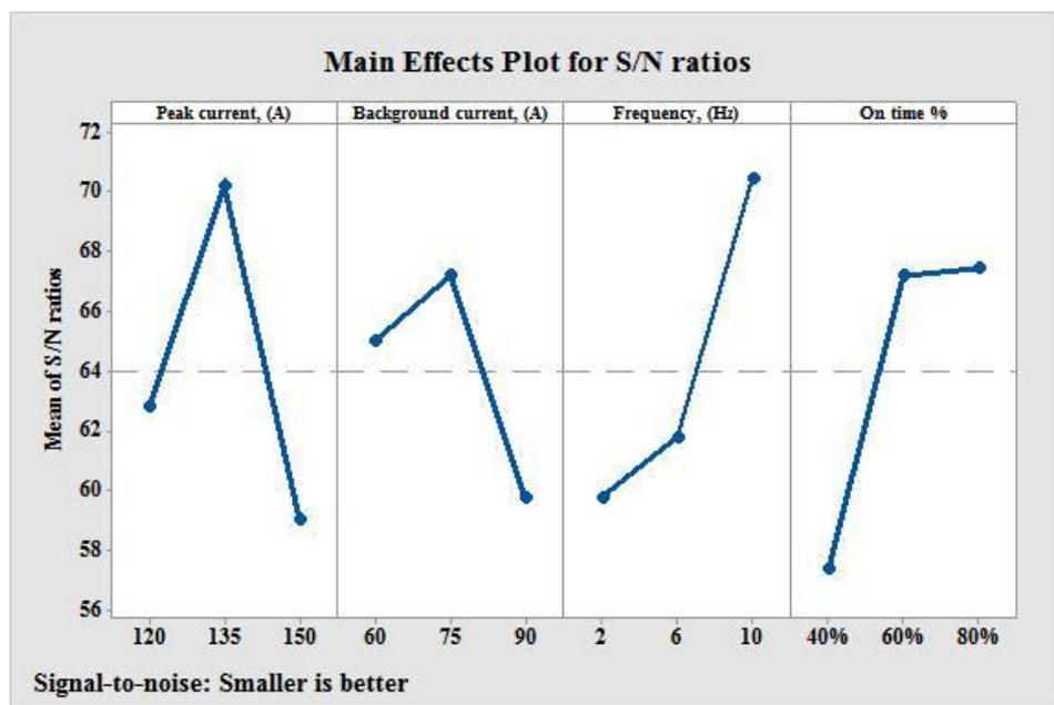
**Fig. 3.** S/N Response graph for corrosion rate.
