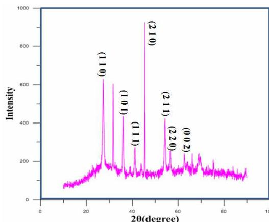
**Fig. 2.** X-ray diffraction pattern of TiO<sub>2</sub> nanorods on the substrate without seed layer
