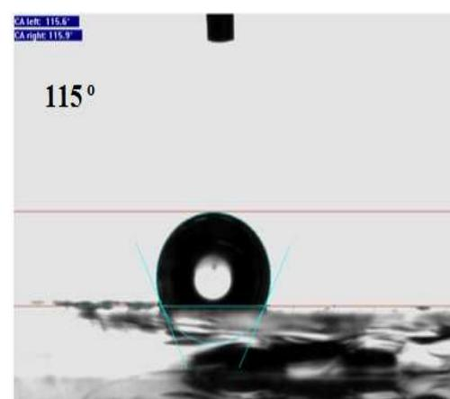
**Fig. 10.** Water drop on top of well-aligned TiO<sub>2</sub> nanorods with 0.1mol concentration (sample C)
