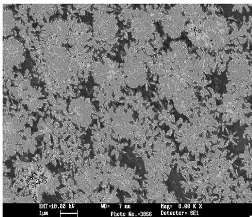
**Fig. 1.** SEM image of TiO<sub>2</sub> nanorods on the substrate without the seed layer
