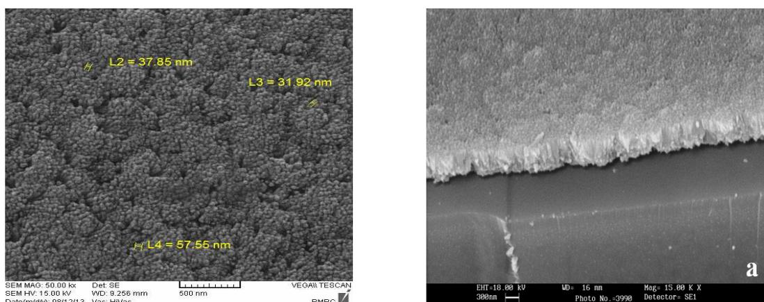
Fig. 6. SEM images of  $\text{TiO}_2$  nanorods with 0.1 mol concentration: (a) cross view, (b) top view
