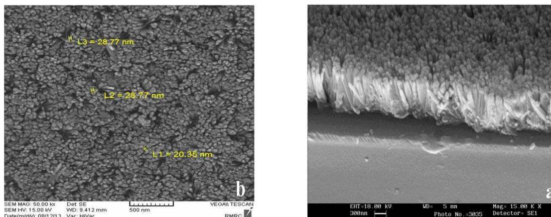
Fig. 5. SEM images of  $\text{TiO}_2$  nanorods with 0.05 mol concentration: (a) cross view, (b) top view
