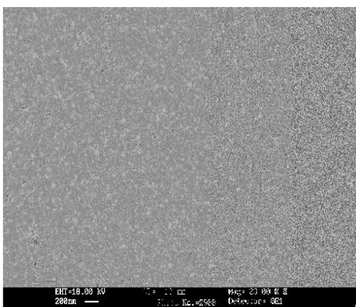
**Fig. 3.** SEM image of the seed layer for TiO<sub>2</sub> nanoparticles which has been annealed at 500°C
