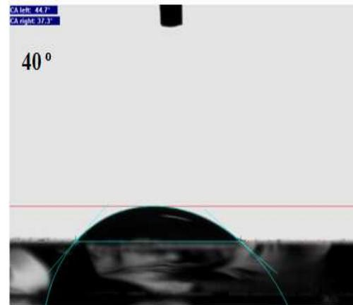
**Fig. 8.** Water drop on annealed TiO<sub>2</sub> seed layer (sample A)
