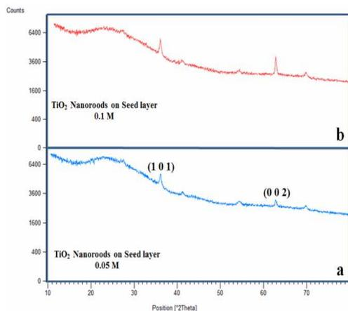
**Fig. 7.** X-ray diffraction pattern of well-aligned TiO<sub>2</sub> nanorods at (a) 0.05 and (b) 0.1 mol concentrations
