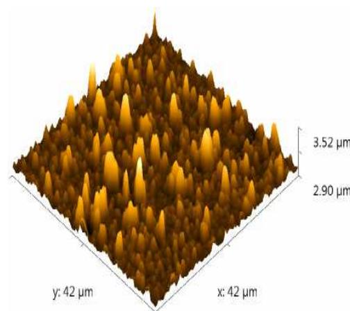
**Fig. 4.** AFM image of the seed layer for TiO<sub>2</sub> nanoparticles
