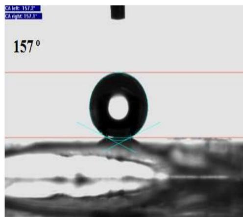
**Fig. 9.** Water drop on top of well-aligned TiO<sub>2</sub> nanorods with 0.05mol concentration (sample B)
