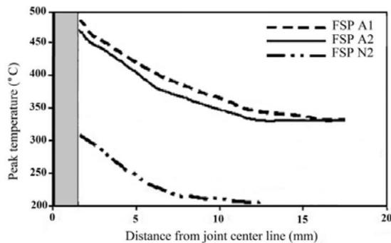
**Fig. 3.** Thermal profile of the FSPed joints, related to the RS
