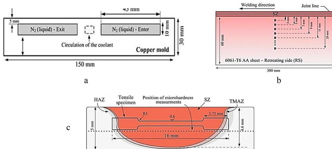
**Fig. 1.** (a) Copper anvil designed as backing plate used for FSP, (b) location of thermocouples with respect to the welding direction and SZ, (c) Schematic illustration of the FSW/FSP cross section, showing the location of the tensile specimens in the SZ and the possible in the central area of the microhardness measurements in the transverse section.
