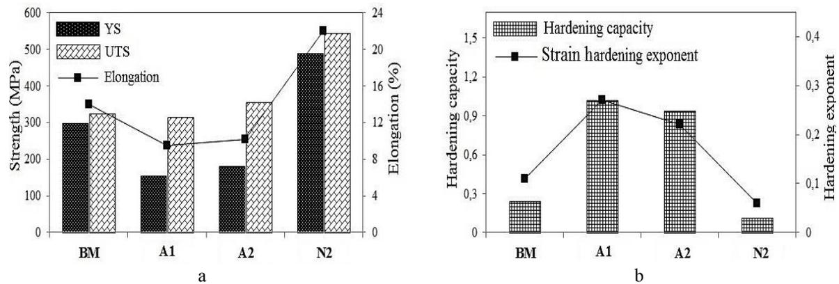
**Fig. 7.** (a) Tensile properties of the BM and FSPed AA 6061-T6 joints (YS: yield strength, UTS: ultimate strength, and El: elongation), (b) hardening capacity and strain hardening exponents
