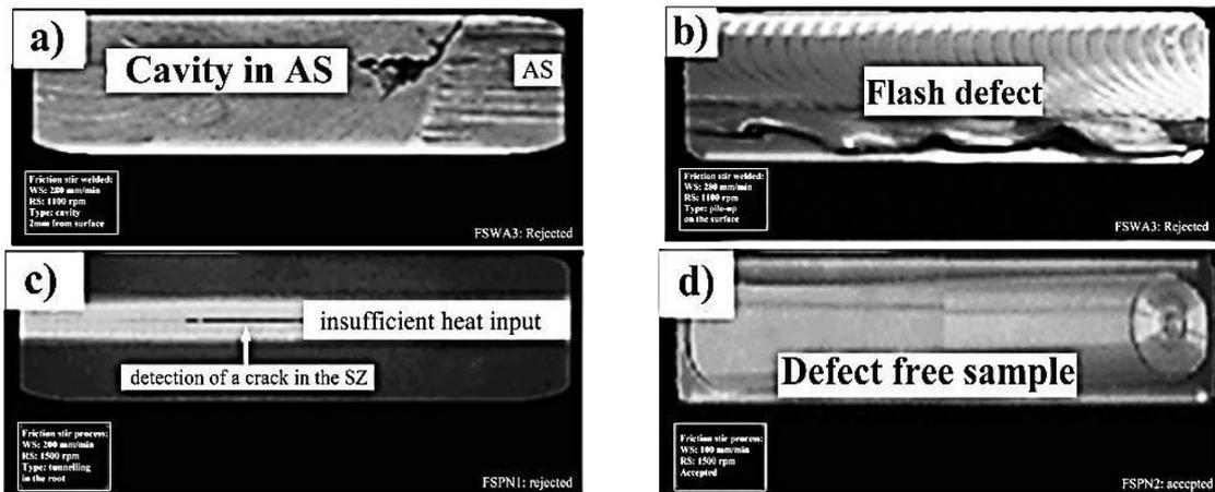
**Fig. 2.** Examples of some representative visual and radiography inspections of the FSWed samples. (a, b) A3: rejected due to formation of a cavity in the AS and flash defect, (c) N1: showing a crack in the root of the SZ of the joint, (d) N2: accepted joint with no macro- and micro-defects
