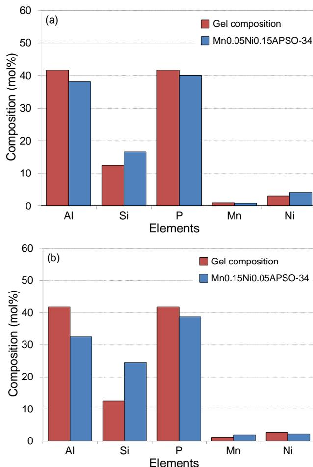
**Fig. 7.** Gel vs. crystal composition of the synthesized nanostructured catalysts: (a) Mn<sub>0.05</sub>Ni<sub>0.15</sub>APSO-34 and (b) Mn<sub>0.15</sub>Ni<sub>0.05</sub>APSO-34
