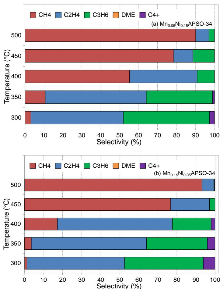
**Fig. 10.** Products selectivity over the synthesized nanostructured catalysts: (a)  $\text{Mn}_{0.05}\text{Ni}_{0.15}\text{APSO-34}$  and (b)  $\text{Mn}_{0.15}\text{Ni}_{0.05}\text{APSO-34}$
