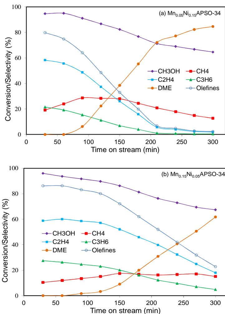
**Fig. 11.** Time on stream performance of synthesized nanostructured catalysts: (a)  $\text{Mn}_{0.05}\text{Ni}_{0.15}\text{APSO-34}$  and (b)  $\text{Mn}_{0.15}\text{Ni}_{0.05}\text{APSO-34}$
