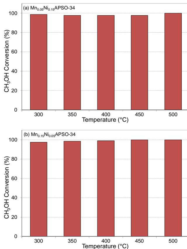
**Fig. 9.** Biomethanol conversion over the synthesized nanostructured catalysts: (a) Mn<sub>0.05</sub>Ni<sub>0.15</sub>APSO-34 and (b) Mn<sub>0.15</sub>Ni<sub>0.05</sub>APSO-34
