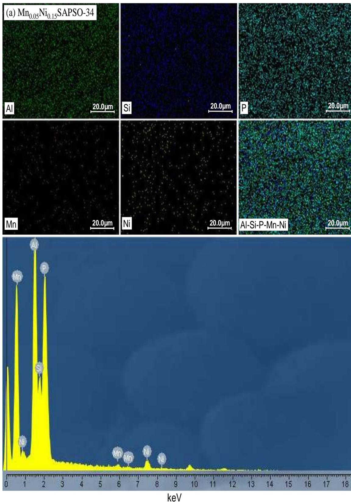
Fig. 6. EDX analysis of the synthesized nanostructured catalysts: (a)  $\text{Mn}_{0.05}\text{Ni}_{0.15}\text{APSO-34}$
