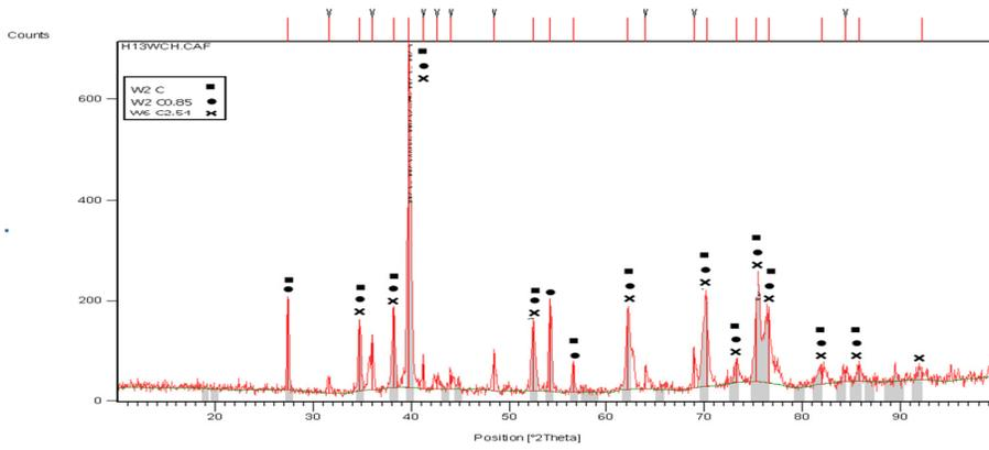
Fig.4. XRD pattern of coating of H specimen.
