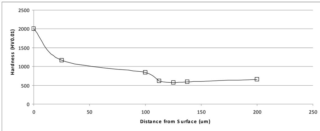
**Fig.8.** Micro-hardness diagram of H and L specimen.
