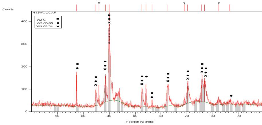
Fig.5. XRD pattern of coating of L specimen.
