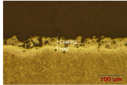
**Fig.9.** Etched cross-section of H specimen, coating & HAZ.
