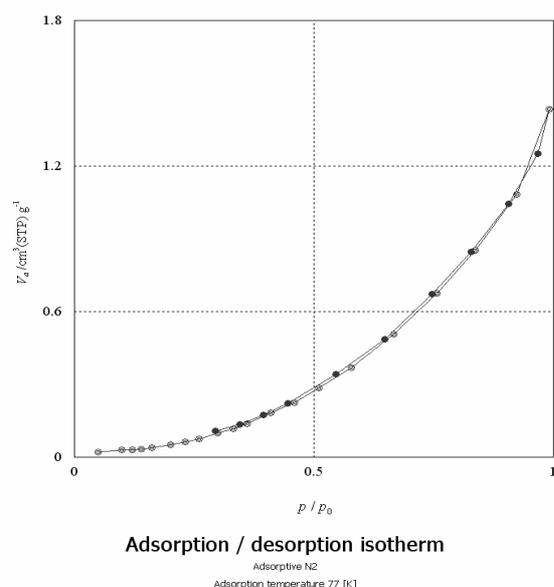
**Fig. 3.** N<sub>2</sub> adsorption/desorption isotherm at 77K of SrFe<sub>12</sub>O<sub>19</sub> nanopowder calcined at 1000°C.
