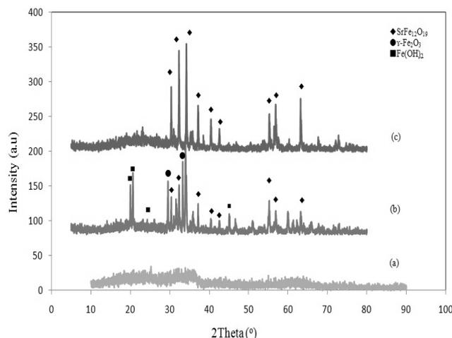
**Fig. 1.** XRD patterns of  $\text{SrFe}_{12}\text{O}_{19}$  nanopowder synthesized via co-precipitation method before (a) and after calcination at  $800^\circ\text{C}$  (b),  $1000^\circ\text{C}$  (c), for 2 h.
