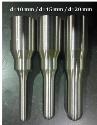
Fig. 2. Vibrating forming tools
