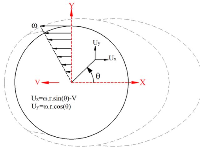
Fig. 1. Detachment of linear and rotational speeds
