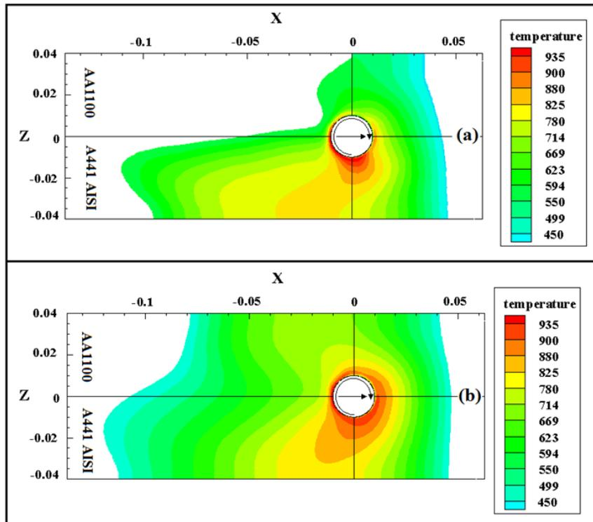
**Fig. 8.** Temperature distribution at the surface of the base metals (a) 10s and (b) 20s after starting welding
