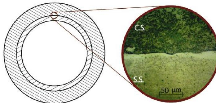
**Fig 5.** OM micrograph of the interface between stainless steel and carbon steel tubes.
