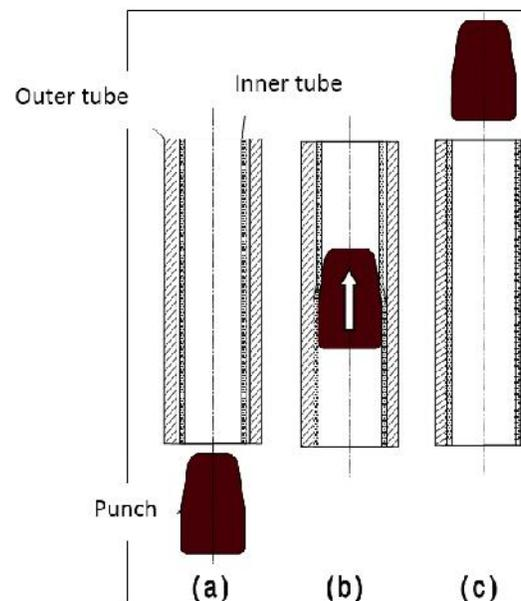
**Fig 1.** Schematic of PPDPC process (a) at the start (b) during deformation of the inner tube (c) cladded bimetal tube at the end of the process.
