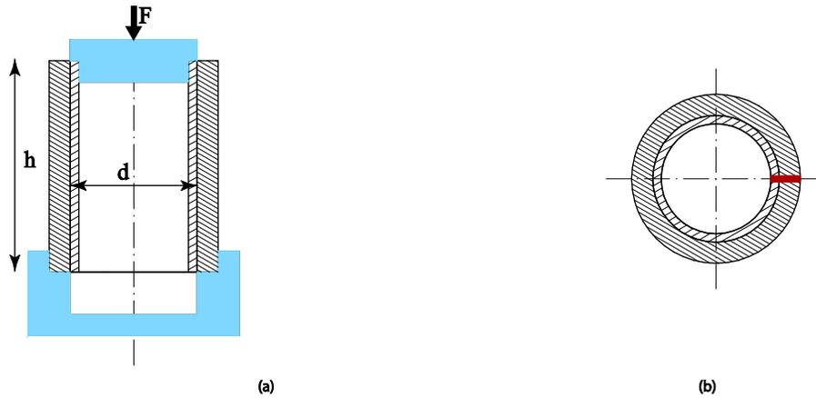
**Fig 3.** (a) Shear punch test tools, (b) microhardness and microstructure measurement position.
