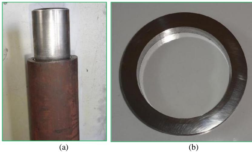
**Fig 4.** (a) A die setup including assembled tubes and process punch at the start of the process, (b) a cross section of processed bimetallic pipe.
