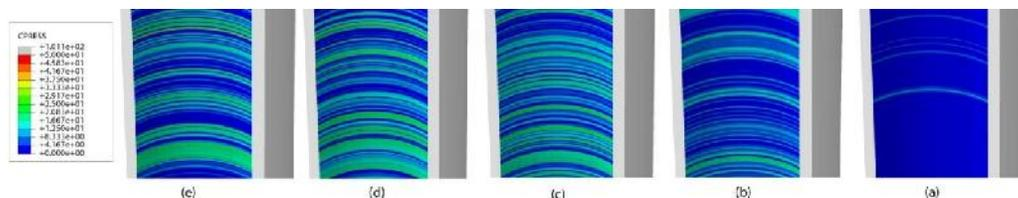
**Fig 9.** (a)-(e) Contact pressure contour between the outer and inner tubes for various inner tubes with inner diameters of 74 mm to 80 mm.
