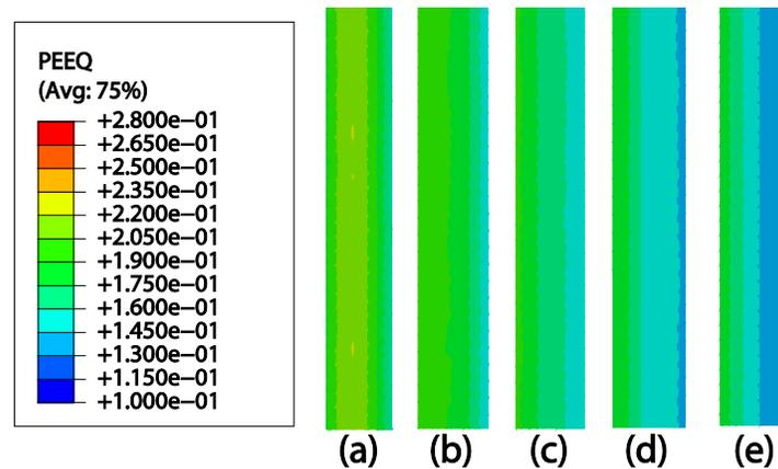
**Fig 8.** Equivalent plastic strain contours of the inner tube in PPDPC process by different punches with punch fillet radius of 20 mm(a), 40 mm(b), 60 mm(c), 80 mm(d) and 100 mm(e).
