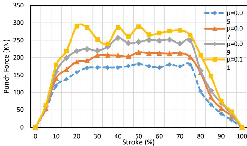
Fig 7. Punch force versus stroke curves in various friction coefficient.
