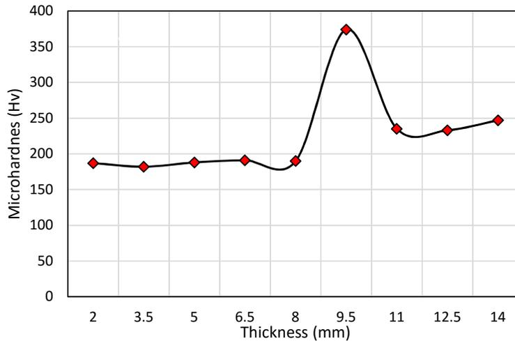
Fig 6. Microhardness variation along the thickness of the processed bimetal tube (left: carbon steel, Right: stainless steel).
