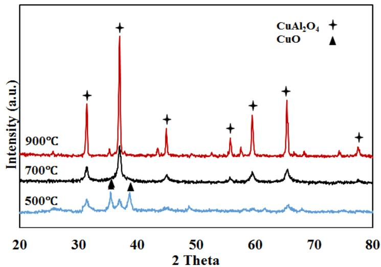
Fig 1. X-ray diffraction patterns of the samples calcined at different temperatures
