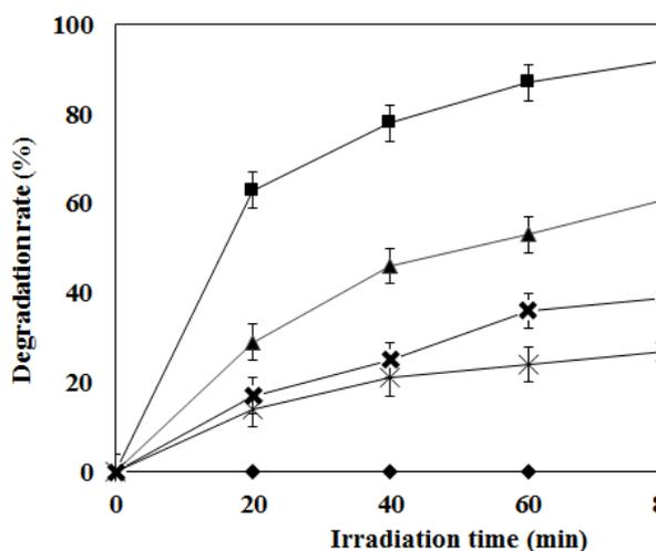
**Fig. 6.** Photocatalytic activity of the samples calcined at different temperatures
