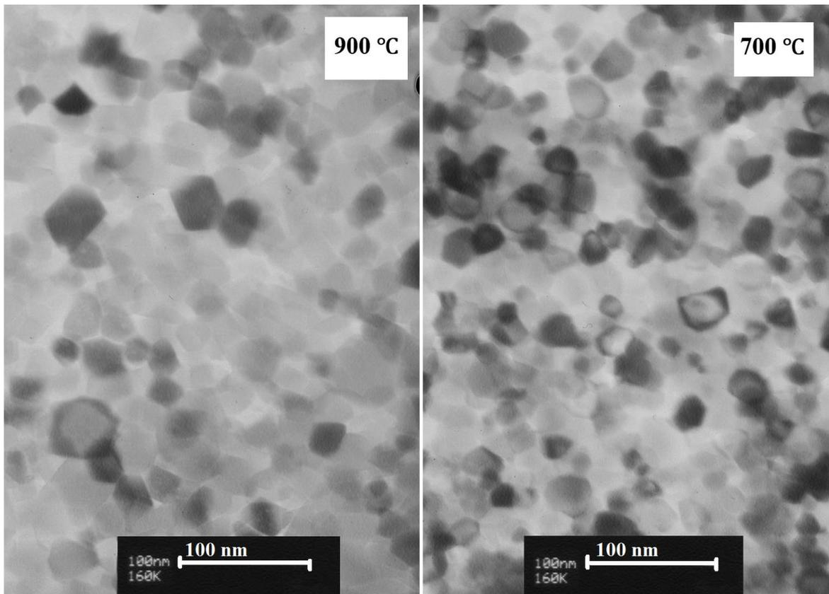
Fig. 4. TEM images of the samples calcined at different temperatures
