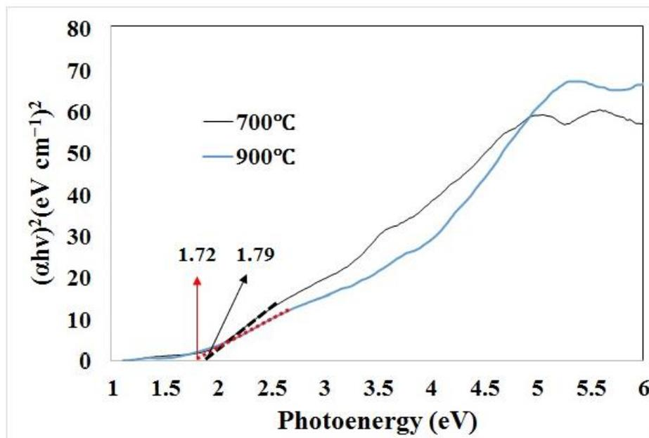
Fig. 5. The plots of  $(\alpha h\nu)^2$  versus photon energy ( $h\nu$ ) of the samples calcined at different temperatures
