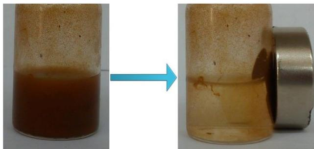
Fig. 1. The process of recovering  $\text{Fe}_3\text{O}_4$ ,  $\text{Fe@B}$ ,  $\text{Fe@B-N}$ ,  $\text{Fe@B-I}$  and  $\text{Fe@B-I-Mo}$  by using a magnet.
