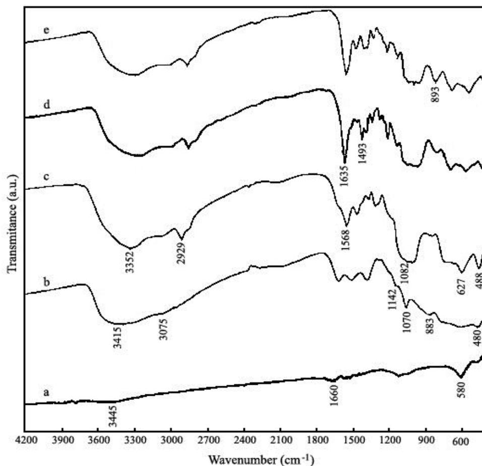
Fig. 2. FT-IR spectra of a)  $Fe_3O_4$ , b) Fe@B, c) Fe@B-N, d) Fe@B-I and e) Fe@B-I-Mo.
