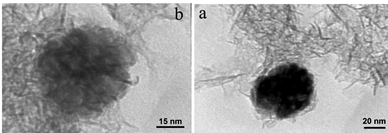
**Fig. 4.** TEM images of a) Fe@B and b) Fe@B-I-Mo.
