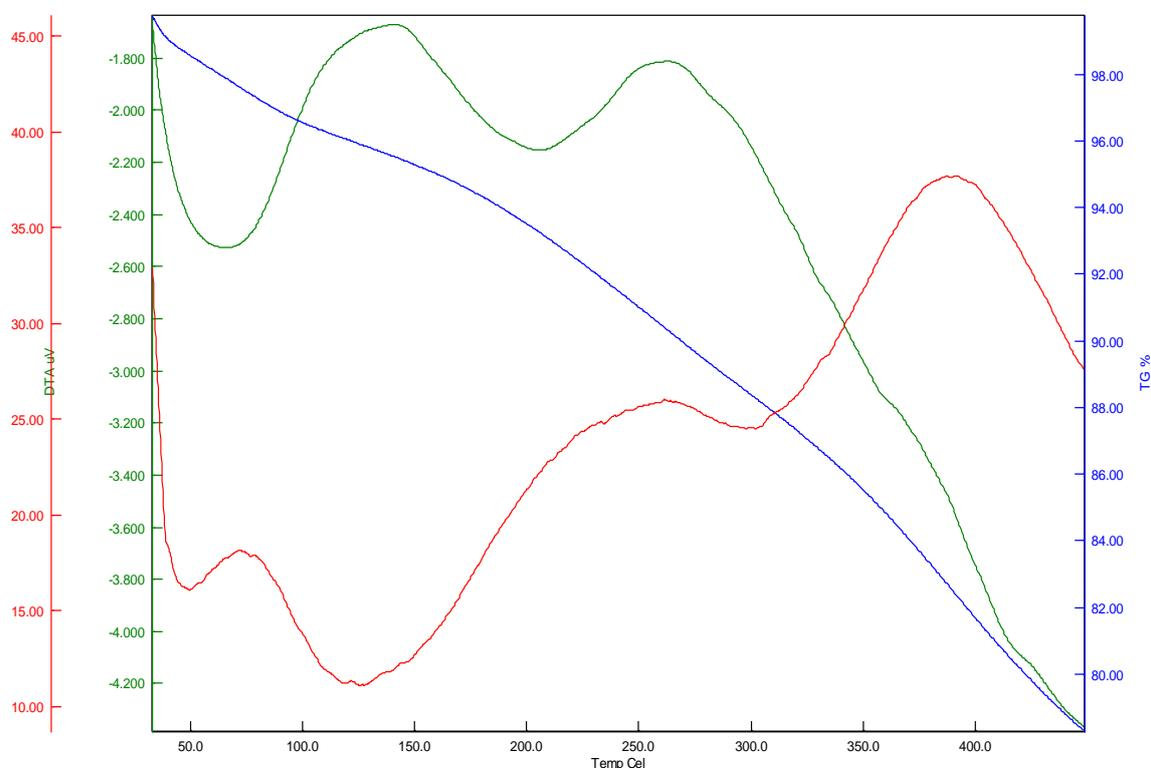
Fig. 5. TG/DTG/DTA thermogram of Fe@B-I-Mo.
