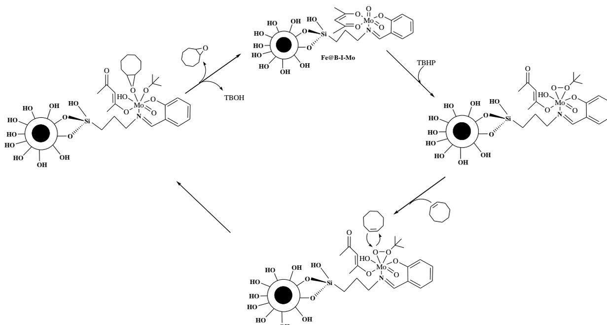
**Scheme 2.** Proposed mechanism for the epoxidation of olefin with TBHP by Fe@B-I-Mo.
