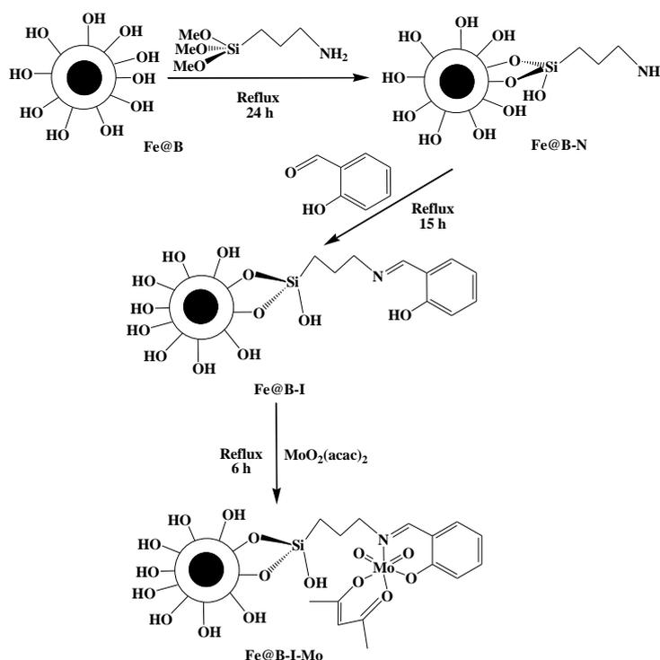
Scheme 1. Preparation of  $\text{Fe@B-N}$ ,  $\text{Fe@B-I}$ , and  $\text{Fe@B-I-Mo}$ .
