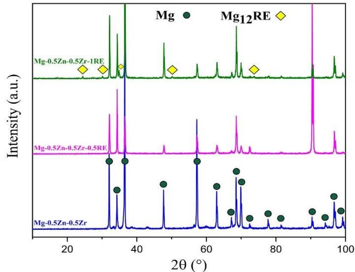
Fig. 3. XRD patterns of as-cast alloys.
