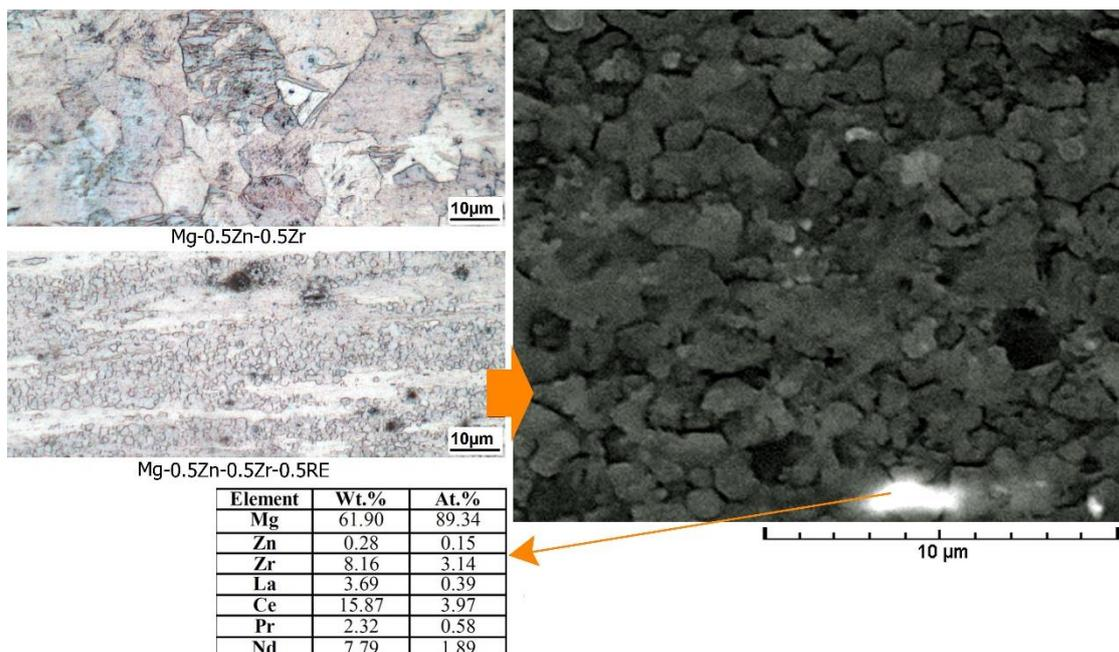
Fig. 4. Optical micrographs of extruded alloys and SEM image of the Mg-0.5Zn-0.5Zr-0.5RE alloy and EDS point analysis of the shown phase
