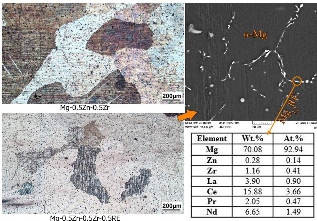
Fig. 2. Optical micrographs of as-cast alloys and the SEM image of the Mg-0.5Zn-0.5Zr-0.5RE alloy and the corresponding EDS point analysis from the intergranular phase..
