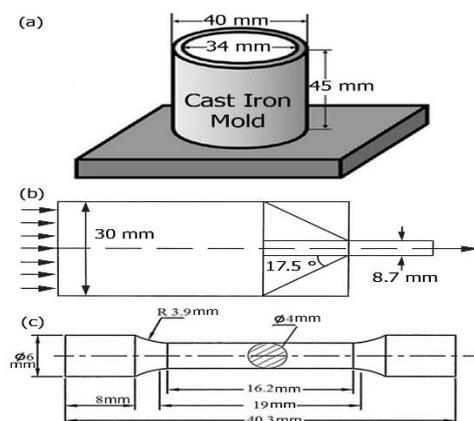
Fig. 1. Details of (a) metallic mold (b) extrusion die, and (c) tensile specimen.
