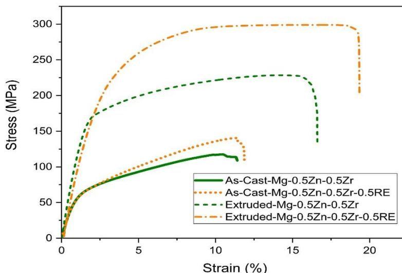
Fig. 5. Representative tensile stress-strain curves.
