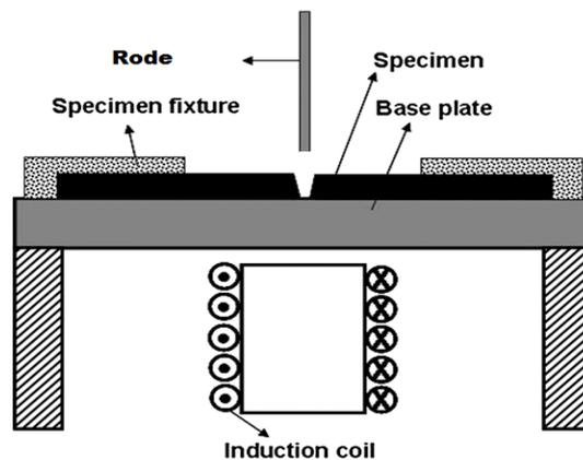
**Fig. 1.** Schematic of the electromagnetic vibration device
