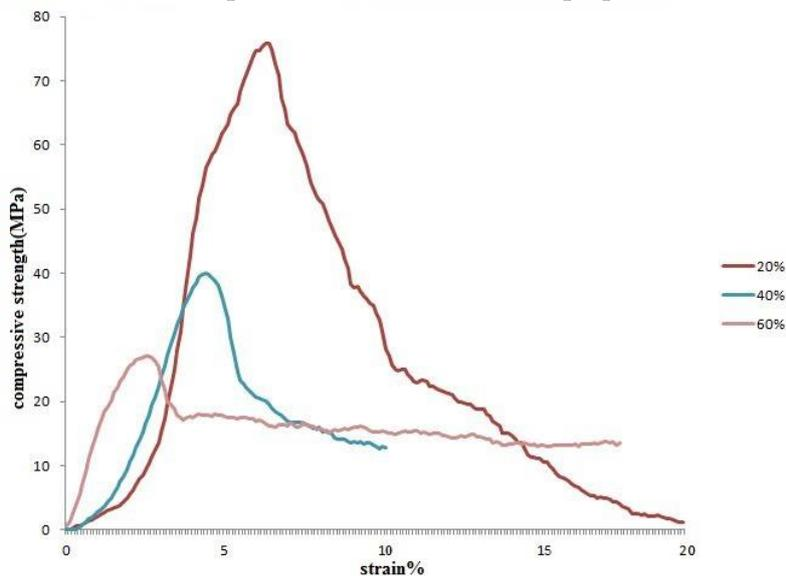
Fig. 8. Compressive stress-strain curves of manufactured FGSs with 20, 40, and 60 Vol.% porosities using urea as space holders.
