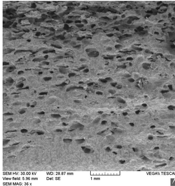
**Fig 5** SEM micrograph of fabricated FGS using Mg as a space holder.
