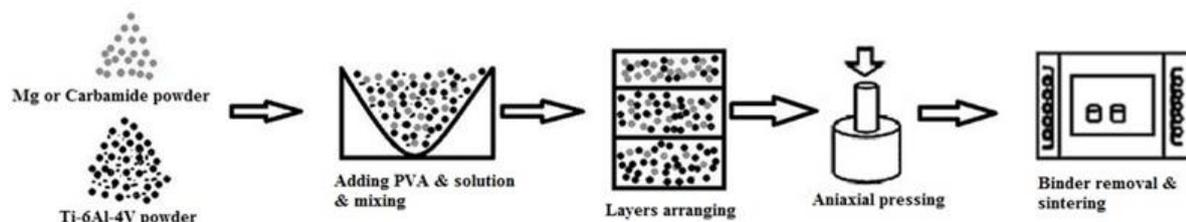
Fig. 1. Schematic of processing steps for fabricating FGSs.
