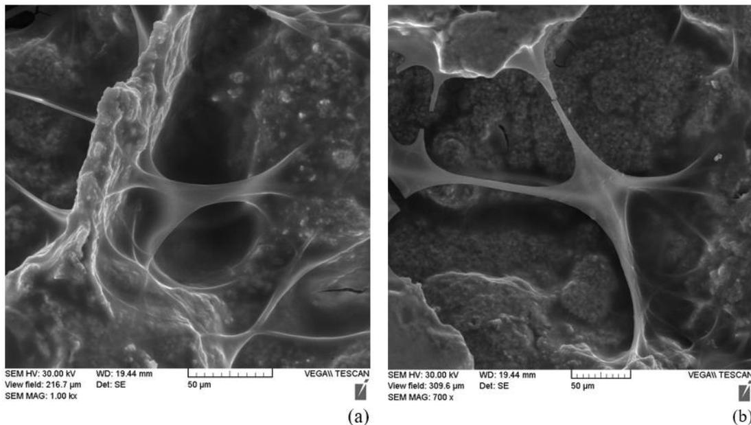
**Fig. 10.** SEM micrograph of MG-63 cells attached to the scaffold's surface using: (a) Mg and (b) Carbamide as space holders after 6 h.
