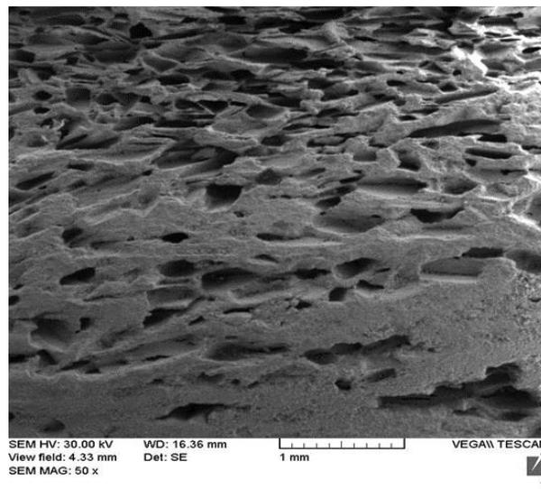
Fig. 3. SEM micrograph of fabricated FGS using urea as a space holder.
