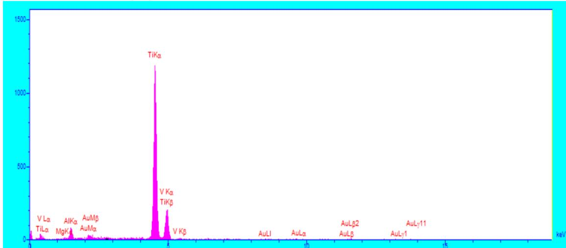
Fig. 7. EDS of fabricated FGS using magnesium as a space holder.
