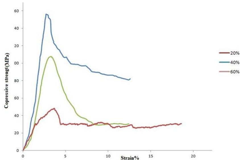
**Fig. 9.** Compressive stress-strain curves of manufactured FGSs with 20, 40, and 60 Vol.% porosities using Mg as space holders.
