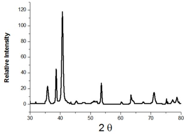
Fig. 2. XRD peaks for fabricated FGS used Mg as a spaceholder.
