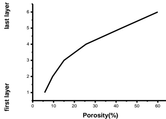
**Fig. 6.** variation of porosity in FGS with Mg as a space holder.
