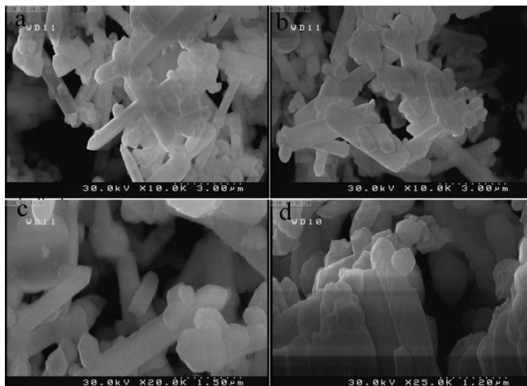
Fig. 3. SEM images of the solid state synthesized  $\text{Bi}_2\text{Mn}_2\text{O}_7$  nanomaterials at 550 °C for 8h
